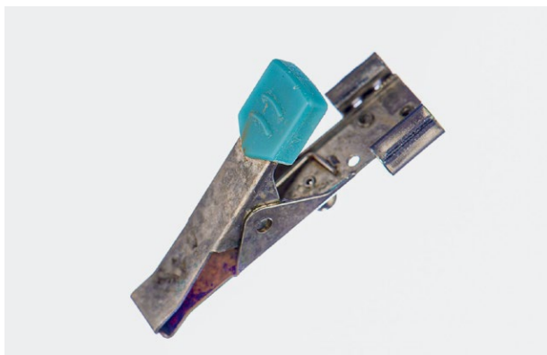
Fig. 7 - Electrocardiogram (ECG) clip damage secondary to excessive use without cleaning between patients and using alcohol instead of ECG gel, which causes faster corrosion of the metal. This clip is rusted and so is the spring, which can cause damage to the patient's skin as well as inaccurate readings.
