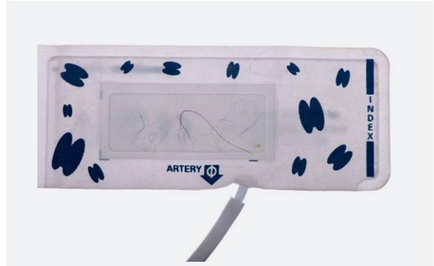
Fig. 5 - Noninvasive blood pressure cuff with hair on the Velcro, making it unable to hold continuous contact. This cuff is dirty and, even after being cleaned, remains discolored. In addition, the hose to this cuff is loose, causing it to have a possible air leak and deliver inaccurate measurements.
