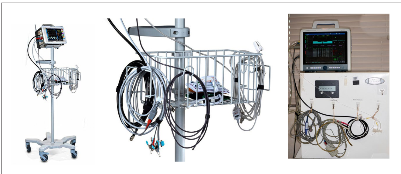
Fig. 8 - Management of peripheral wires after use; a) rolling stand with coiled wire storage (Digicare); b) close-up showing hooks; c) wires attached with wraps on lift table.
