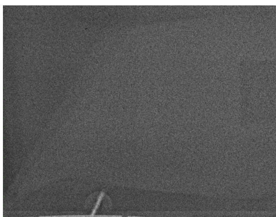
Figure 1: Note the marked generalised increased image darkening, as result of multiple small grey opacity speckles on the imaging plate. There are also patterns seen within the image, because the cassette was stored behind an unknown object when radiographs were made.
